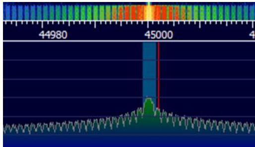
• Spectrum with square bits is very wide and shows the characteristic sinc shape in the frequency domain
